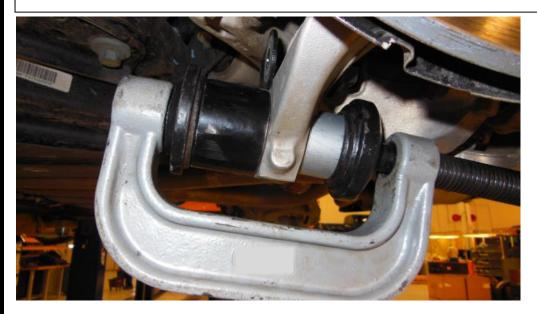
9.3 Press in new bearing and ensure bearing is centered in knuckle. NOTE: Use Red Loctite on bearing mating surface.
